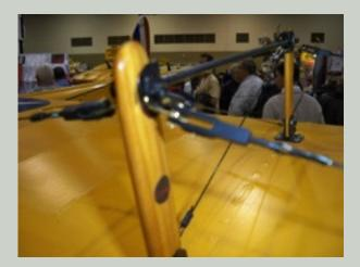
This Curtis JN-4D Jenny was masterfully built by Randy Charles of Wilmington, Ohio. Note the hand made leather straps, and the detail of the hand made turn buckles and guy wires. (built in less than six months!!!!!)
